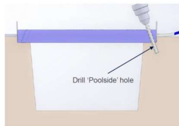
Fig 4 - Drilling using Drilling Template
