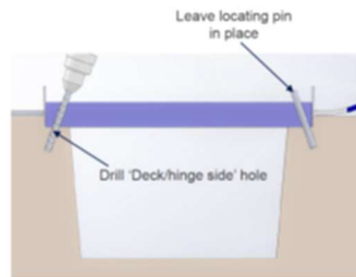
Fig 6 - Drilling using Drilling Template
