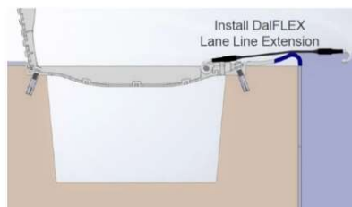
Fig 10 & 11 - DalFLEX Lane Line Extension Installation
