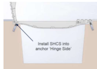
Fig 9 – insert SHCS into DalFLEX hinge side
